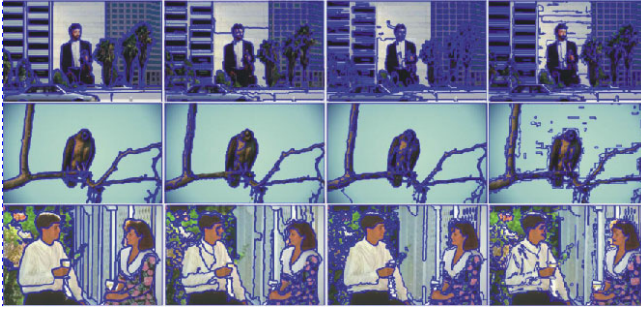
Fig. 3. Examples of images segmented. From left to right: Human segmentation, Our segmentation, Mean-Shift segmentation and Local Variation segmentation.
